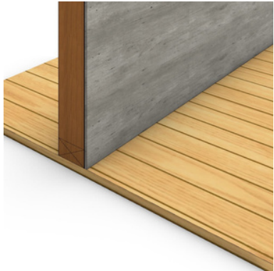
Floor Junction on Framing
