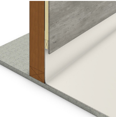
Floor Junction with Batten and Vinyl
